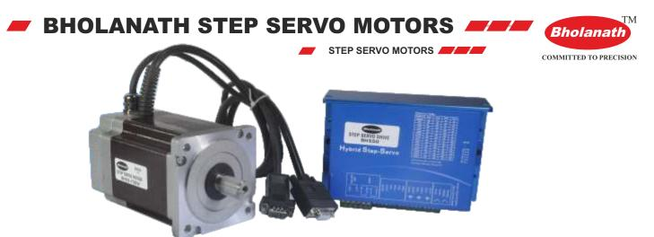
Bholanath Step Servo motors are closed loop stepping systems - high speed (>2000 RPM) stepper motors with incremental optical encoders and digital drives.
